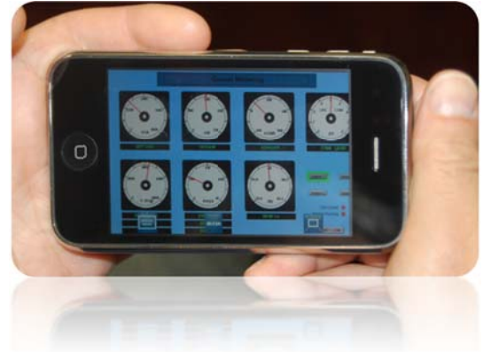
Figure 6: Secure Remote Access to Operator Station allows users to access the "Virtual Switchgear"
