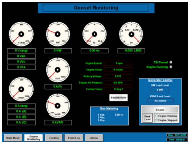
Figure 1: APTView Genset Monitoring and Control
