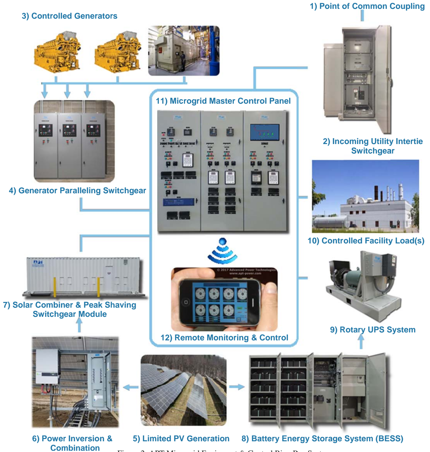
Figure 2: APT Microgrid Equipment & Control Ring Bus System
