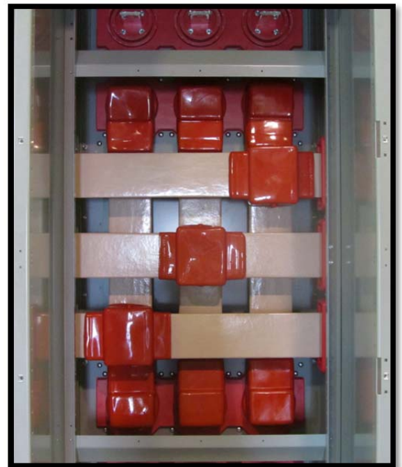
Figure 7: Main bus is insulated silver plated copper, with bolted connections covered by insulating boots.
