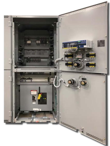
Figure 3: 15kV Max Controls Cubicle over Vacuum Circuit Breaker Metal-Clad Section
