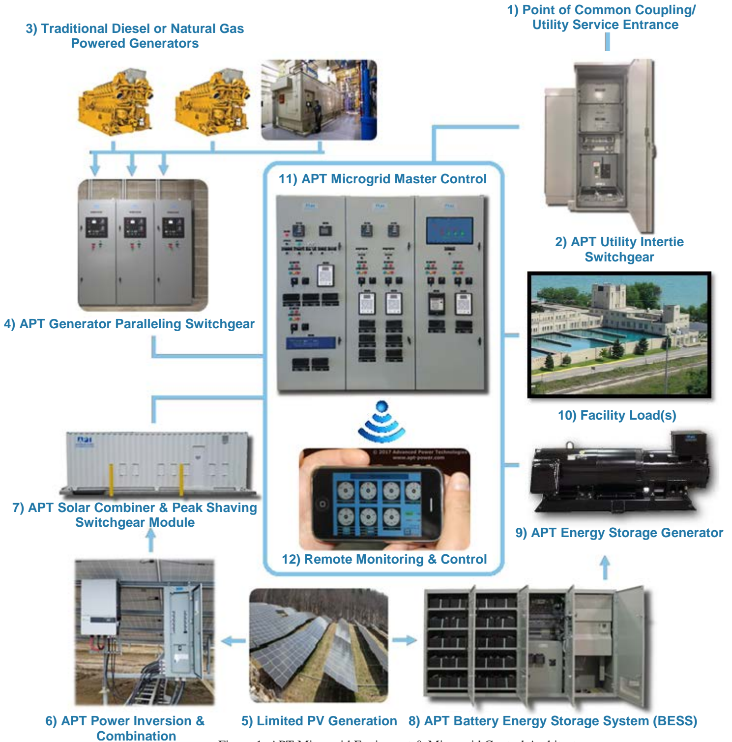
Figure 1: APT Microgrid Equipment & Microgrid Control Architecture
