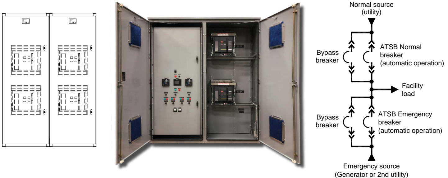
Figure 23: UPS Bypass/Isolation Maintenance Switchboard*
