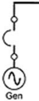
Figure 9: Single Generator Disconnect & Output Protection
