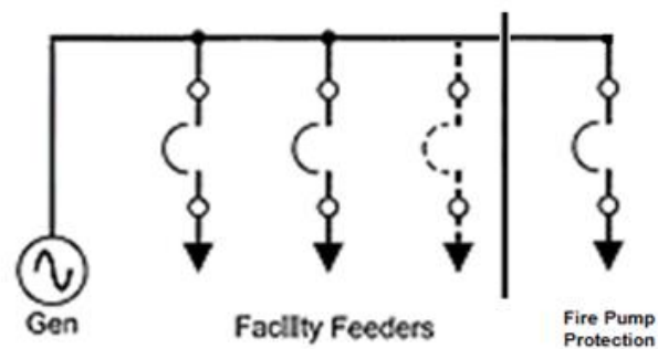
Figure 20: Single Generator Disconnect/Output Protection with Distribution Feeders, & Fire Pump Protection
