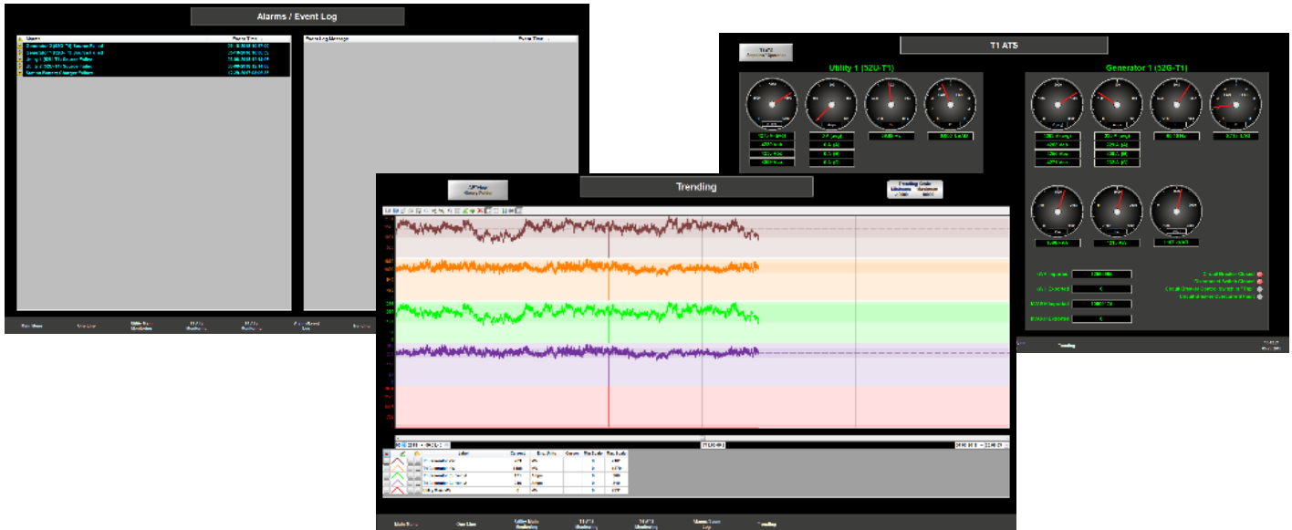
Figure 8: Event Log (top left), Source Metering Data (top right), Power Usage Time Adjustable Trend Chart (bottom)
