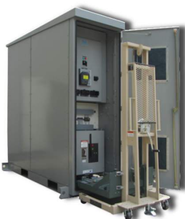
Figure 16: Lift truck pushed toward the circuit breaker cell so cradle is square for removal
