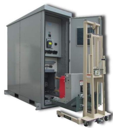
Figure 18: Cradle raised to clear the blocks on each side of the circuit breaker cell rails
