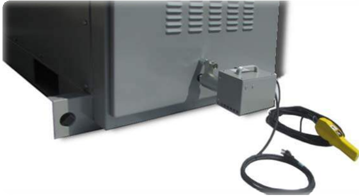
Figure 9: Electric Racking Device with cable to accommodate remote racking of the circuit breaker up to 50 ft. away
