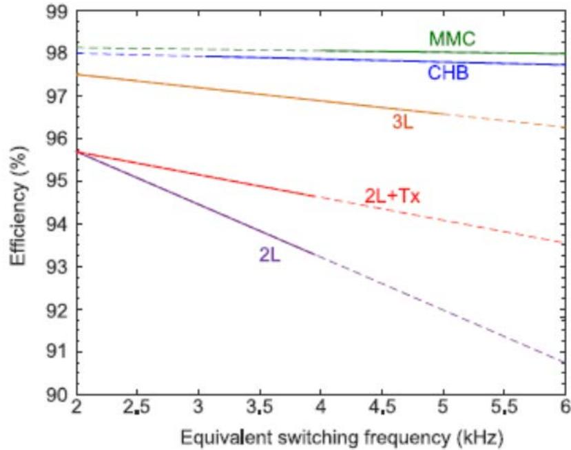
Fig. 6 Efficiency of compared configurations at various equivalent switching frequencies with the power level of 0.8 pu.
