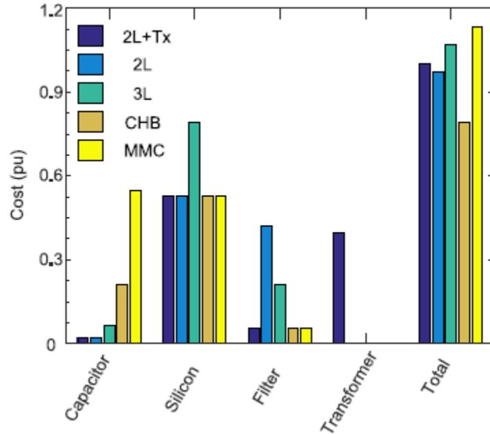
Fig. 10. Cost Breakdown per Component for Each Topology Per Unit Cost
