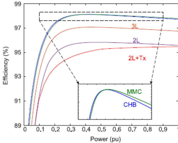
Fig. 7 Efficiency of compared configurations at various power levels.
