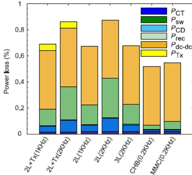
Fig. 8 Breakdown of entire PE unit losses for different configurations at 10% load.
