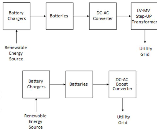
Fig. 1. Functional Block Diagram of Transformer Based BESS Topology (top)
