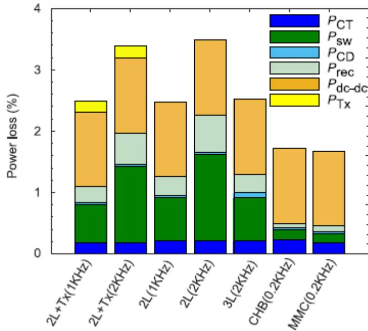
Fig. 9 Breakdown of entire PE unit losses for different configurations at 80% load.
