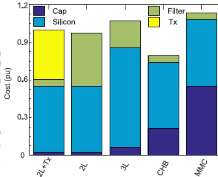
Fig. 11. Cost Breakdown per Topology for Each Component Per Unit Cost
