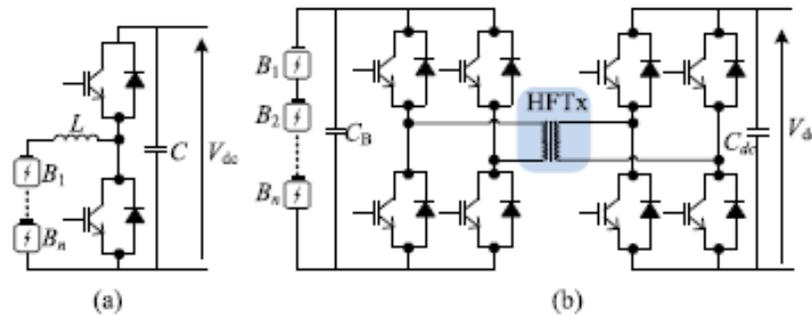
Fig. 4 Common dc-dc converter topologies to control the power flow between the common dc-link and batteries, (a) boost converter, and (b) DAB converter.
