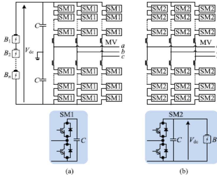
Fig. 3 MMC and corresponding SMs: (a) centralized batteries on the dc-link; (b) distributed batteries in the SMs.
