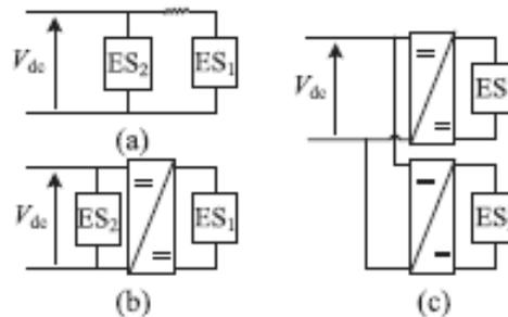
Fig. 5 Typical categories of configurations to connect multiple ES resources: (a) direct connected; (b) half controlled; and (c) fully controlled.
