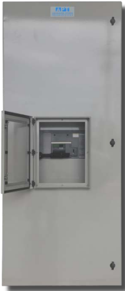
Figure 1: 1.3MW, 480V, 2000A Generator Disconnect & Output Protection Molded Case Circuit Breaker NEMA 1 Enclosure with Window Kit
