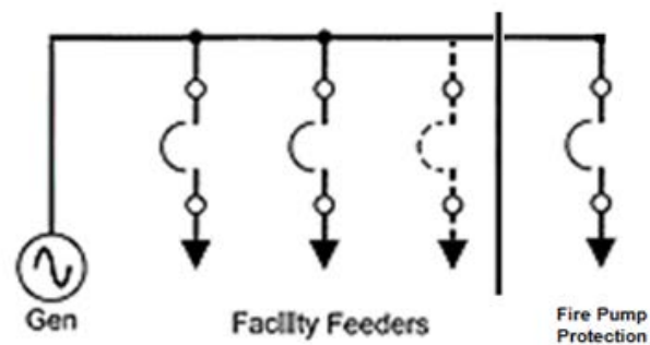
Figure 22: Single Generator Disconnect/Output Protection with Distribution Feeders, & Fire Pump Protection
