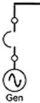
Figure 9: Single Generator Disconnect & Output Protection
