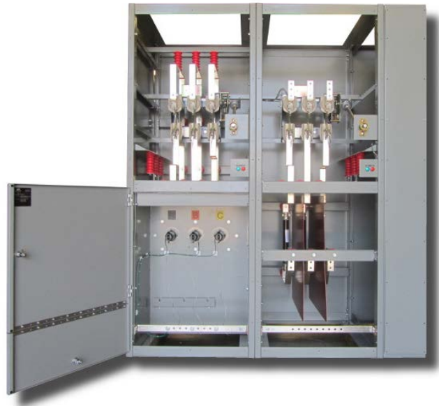
Figure 2: Generator Quick Connection Switchgear MF2-T Series Dual Loadbreak Switch with Overcurrent Protection
