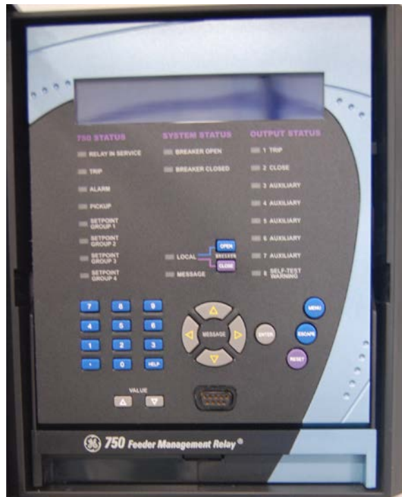
Figure 3.5: SR750 Protection Relay
